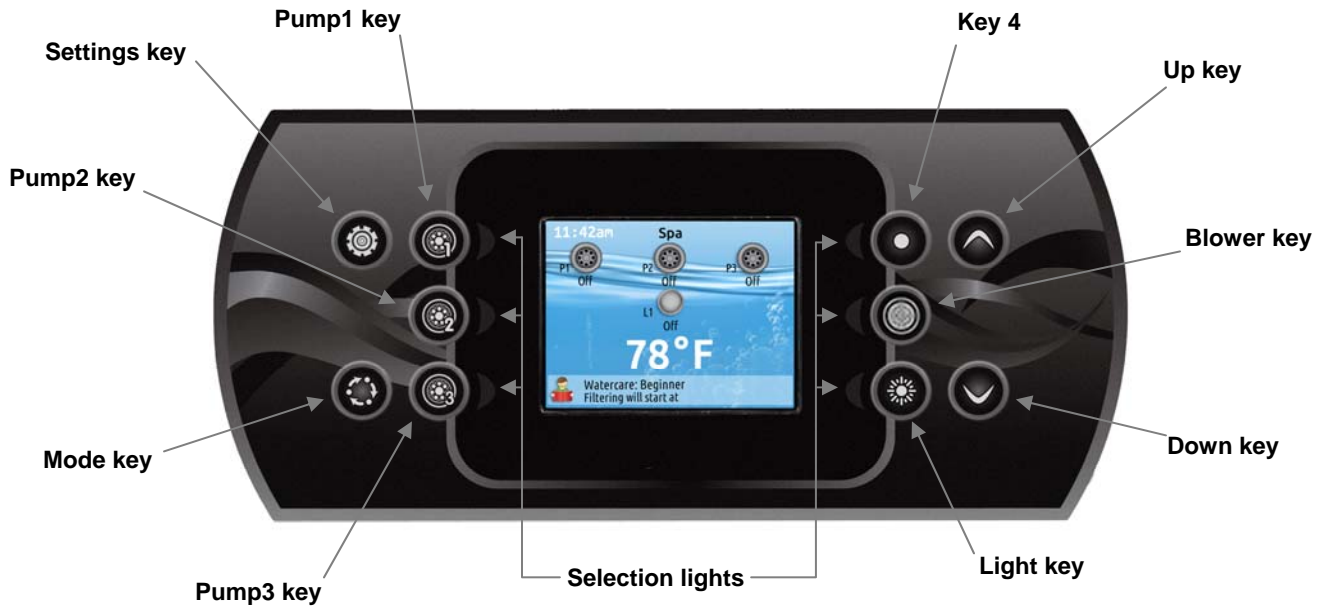
in.k806 Control Panel
